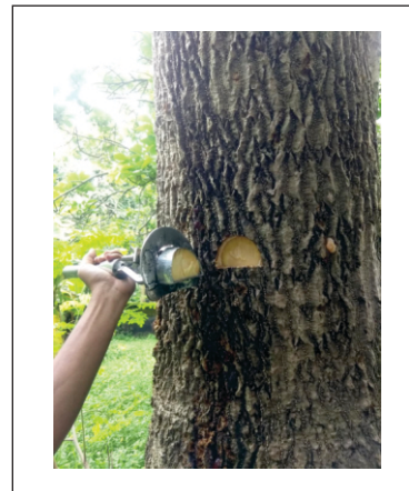
Fig. 6: Blaze development using gum tapping blazer
