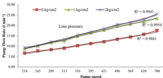
Fig. 4: Pump Flow rate affected by speed and line pressure
