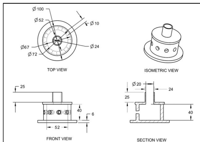
Fig. 1: Different views of the cylindrical fertilizer distributor
