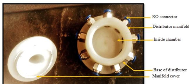
Fig. 2 : Different parts of Liquid fertilizer distributor
