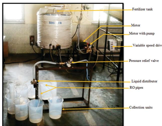
Fig. 3: Experimental set up for evaluation of liquid fertilizer metering
