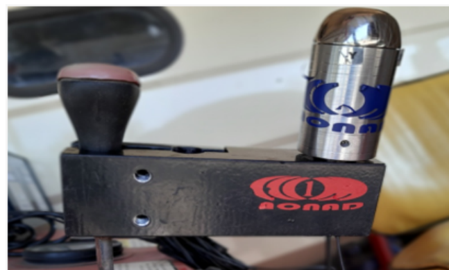
Fig. 3: Measurement of actuating force of gear shifter lever using gear effort sensor
